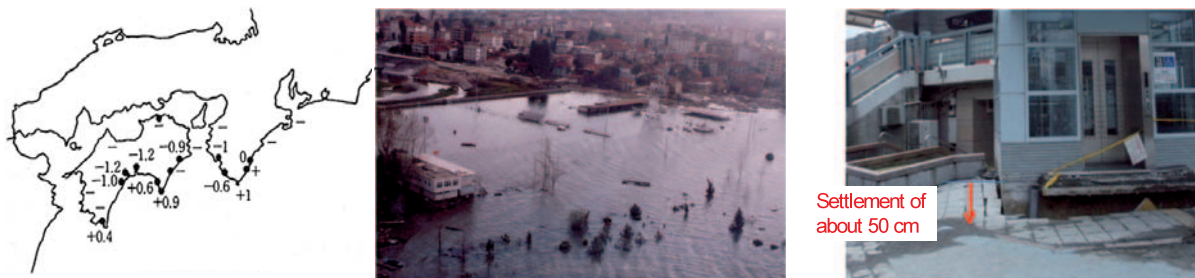
Fig. 10 (left) Ground subsidence and heaving (in meter) by the 1946 Nankai Earthquake (Kawasumi, H.)
