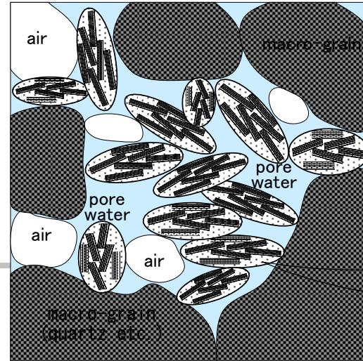
Schematic diagram of bentonite
