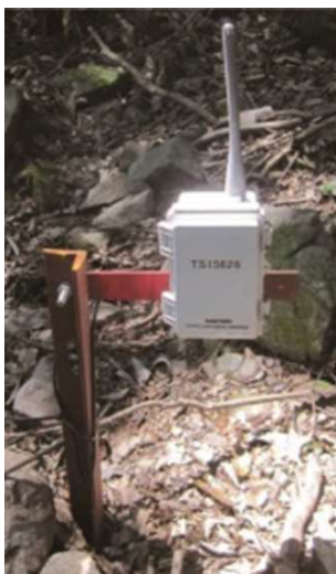
Figure 9 Low-cost monitoring of slope that is prone to rainfall-induced landslide: geotechnical engineering for the people
