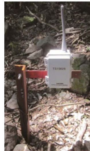
Figure 8 Low cost monitoring of slope prone to rainfall-induced landslide: geotechnical engineering for the people
