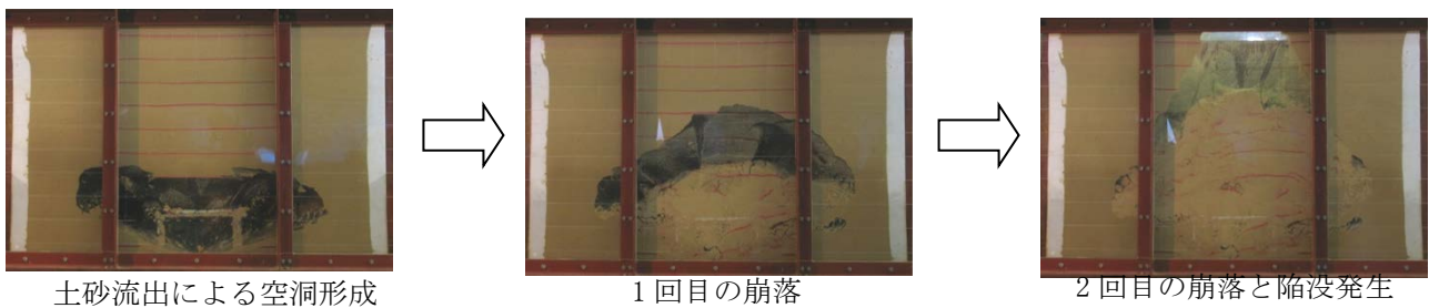
Fig. 1. Collapse of the cavity
