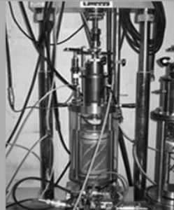
Cyclic Triaxial Test of Soil ( Liquefaction Strength · Deformation Characteristics )
